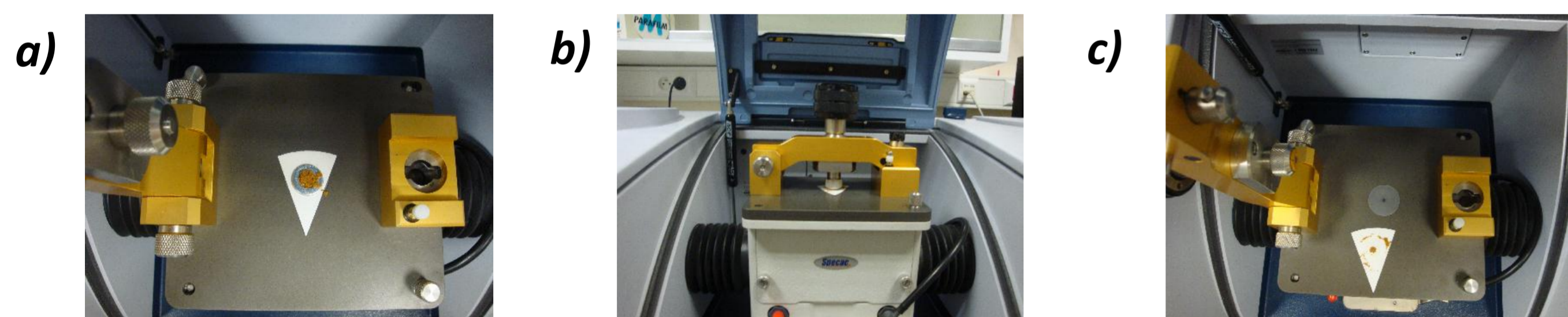
Figure 1: a) Sample preparation on paper filter, b) Fat extraction using the Golden Gate ATR press during 3 min, c) FTIR Analysis of the fat on the diamond ATR (3 replicates)
