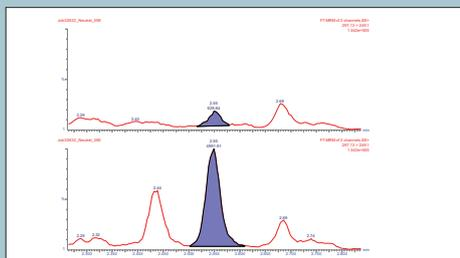
DON analysis: MS/MS chromatograms for DDGS unspiked (top) and DDGS spiked with DON (at 250 µg/kg) before extraction (bottom)
