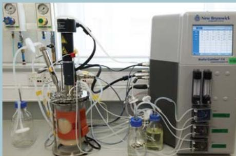
The mycotoxin levels in the inoculated wheat samples will be compared with the levels following fermentation. A laboratory scale fermentor has recently been commissioned and will be used to carry out these studies. Using inoculated wheat samples means that the mycotoxins and other possible new conjugates should be present at high enough levels to be easily measured and to allow mass balance studies to be conducted.
